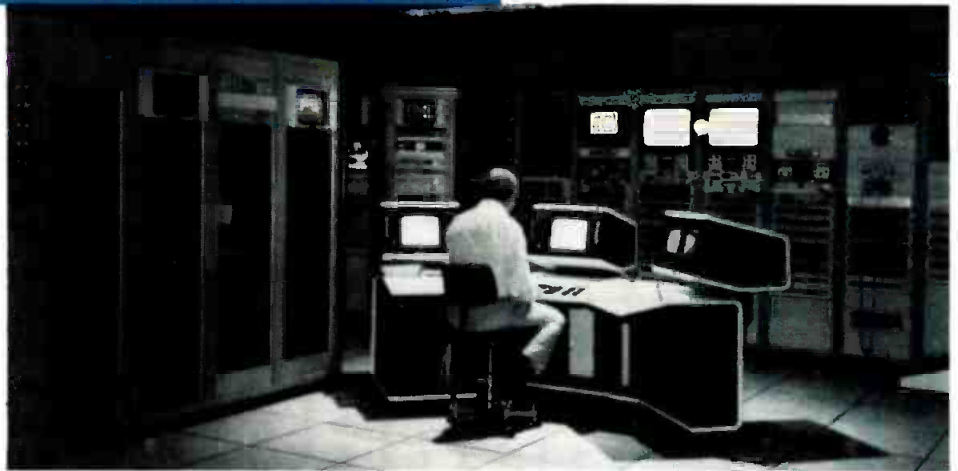
The Thomson Vidifont Graphics V system is located in the center of the master control room. Remote keyboards for the system are located in the editing suites.
