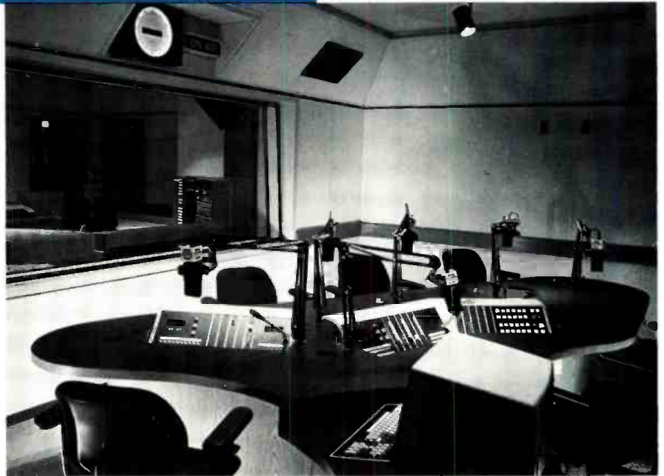
Both Studio 1 (top) and its adjacent control room (below) contain Colorgraphics/Integrated Technology news computers and McCurdy customized talent consoles with intercom and monitor select built in.
