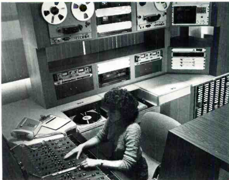
Operating engineer in air control room works on Neve custom console with MCI tape recorders, ITC Delta cart players and Technics turntables in the background.
